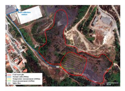
**Figure 3.** General view of the active combustion area in S. Pedro da Cova waste pile and schematic representation of the optical fiber system installation in the field (base map source: Google Earth ©2016 Google Image Landsat Data SIO, National Oceanic and Atmospheric Administration (NOAA), U.S. Navy, National Geospatial-Intelligence Agency (NGA), General Bathymetric Chart of the Oceans (GEBCO)).
